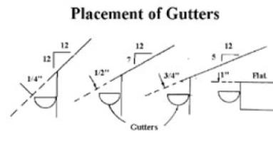
Note: Gutters should be placed below the slope so that snow and ice can slide clear. Steeper pitch requires less clearance.
